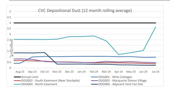
A 12-month rolling average of depositional dust concentrations has been presented above. Dust Gauges DDG001, DDG002, DDG003 and DDG004 are located within a closer proximity to Chain Valley Colliery and DDG006 is positioned in a location representative of the Chain Valley Colliery ventilation fan site at Summerland Point.
